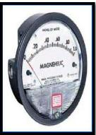
We need Three stage Filtration of Air intake air, daily cleanable V type filter, weekly cleanable one inch depth thick mesh filter embedded on the hood, and next is the real air intake paper filter fitted on compressor mouth suction. The Magnehelic Delta P gauge to measure Air intake filter Delta P to fix on hood, to be monitored daily and keep Pascals minimum.
