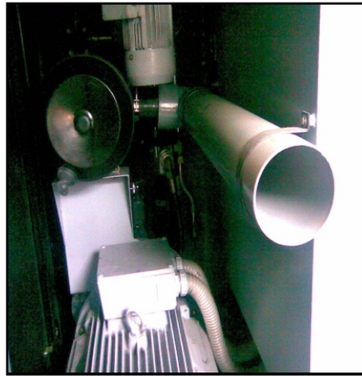
Fig 5. Pre-filter to existing Air intake Filter, pipe Extension to Air Entry. Fig 1. Invest in Air Receiver - / Tail End model
