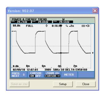
COMPRESSOR LOAD KW = 50.6 KW
